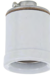
47712- E26, 660W-250V, Keyless glazed porcelain med. base beaded body socket w/flange, 1/8 IPS cap w/set screw, nickel plated copper screw shell, 1 5/8" O.D. x 2 1/4" height, fits clamp type holders
