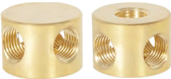
21253U - Brass straight disc arm-back, 1/4F bottom hole, 1 side hole tapped 1/4F , 1 1/4" diameter x 7/8" height, unfinished brass
