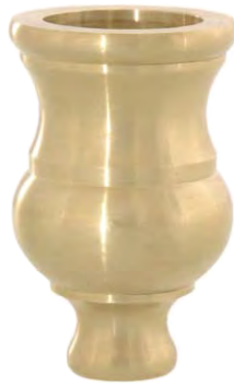
21800U - Unfinished Die Cast Brass Candle Cup, 2 3/8" ht., 1 1/2" O.D., 1" inside top opening. mounts standard or candelabra candle cover, tap 1/8F.
