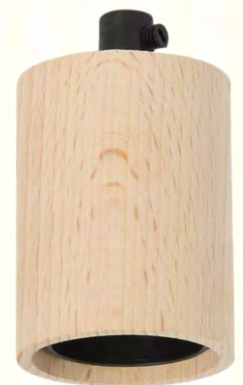
48733 - 2 5/8" tall x 1 5/8" inside diameter unfinished beech wood socket cover with center hole that slips 1/8 IP and comes COMPLETE with E26 quick-connect, medium lamp socket, black nylon cord bushing, and hardware kit (see above) for pendant mounting application.
