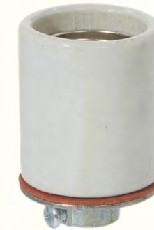
48126i- Keyless glazed porcelain medium base (E26) socket, 1/4 IPS metal cap with set screw, nickel plated copper screw shell, 1 1/2" O.D. x 2 1/16" height, 660W-250V
