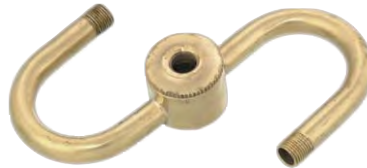
10407U - Unwired S-type, 2-Arm lamp cluster - solid brass. 5 1/4" across body 1/8F (IPS) top X 1/8F bottom, 1/8 male IPS arms. Unfinished brass
