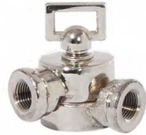
20536N - Die Cast Brass Swivel without teeth and solid brass key. 1 3/4" long x 1 11/16" tall x 1" wide, tapped 1/8F X 1/8F, polished nickel finish
