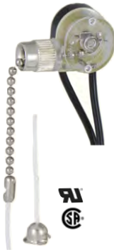
40405N - On-Off pull switch for canopy or fan light, single circuit with nickel finish chain, 6" 18 gauge leads, white cord & bell, rated 3A-250VAC, 6A-125VAC
