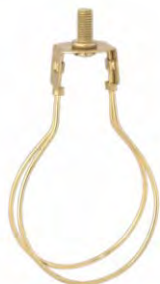
22114 - Shade Adapter. Brass finish. Converts washer type shade to fit on regular shape bulb. 1/4-27M.
