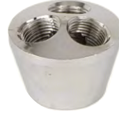
10439N - Nickel Plated, Turned Brass modern tapered body, 3/4" tall X 1 1/8" top diameter, tap 1/4F bottom and 1/8F 3 top holes , nickel plated brass
