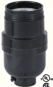
47680- Long Keyless socket, 1/8IP cap With Set Screw , with UNO threads, 660W-250V, 3-piece set, w/screw terminals
