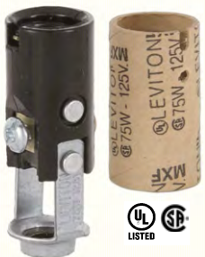
48217 - E12, 75W-125V, Phenolic candelabra base Keyless socket has hickey with 3/4" ht. and 1/8F base. 2 1/16" overall ht. U.L. & C.S.A. listed. LEVITON Brand
