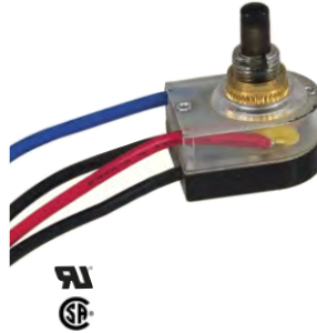
40410 - On-Off Lighted Push canopy switch with black plastic knob & brass finish knurled nut, \frac{3}{8} " metal shank, 6" 18 gauge leads, 3A-250VAC, 6A-125VAC, 6A-125VAC, 6A-125VAC
