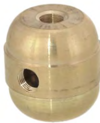
Large turned Brass 2-pc. cluster body - UNFINISHED BRASS Ht. 1 5/8", Dia. 1 1/2" Top 1/8F; Bottom 1/8F 10450A - 2 side holes 10451A - 3 side holes 10452A - 4 side holes 10448U - 5 side holes 10453U - 6 side holes All with 1/8F side holes
