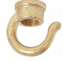
21248U - 1 1/16" tall x 1 3/32" diameter rounded hook with wire way, tap 1/8F through, unfinished
