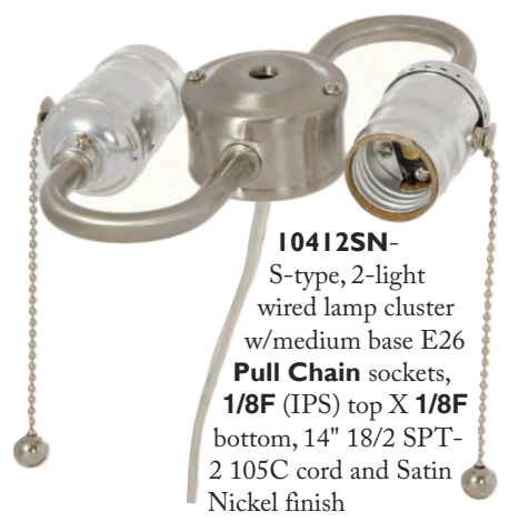
S-type, 2-light wired lamp cluster with medium base E26 Pull Chain sockets, 1/8F (IPS) top X 1/8F bottom, 14" 18/2 SPT-2 105°C lamp cord. Choice of finish. 250W-250V 10412N - Nickel plated finish, clear silver cord 10412 - Brass plated finish, clear gold cord
