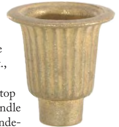
11525U - Stamped brass candle cup, 1" tall x 1 1/2" O.D. x 1 1/8" I.D., slips 1/8IP. Unfinished
