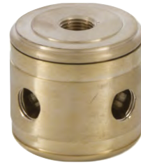
10437 - Turned Brass 2-Piece Modern Cluster Body, 1 1/2" diameter, 1 1/4" height, Top & bottom tapped 1/8F, 4 side holes tapped 1/8F, unfinished
