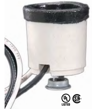
48117- E26, 660W-250V, Porcelain unglazed medium base Keyless socket with 1/8 IPS hickey, two 9" leads rated 18 AWG 105°C, & copper alloy screw shell. Rated for indoor applications. LEVITON Brand
