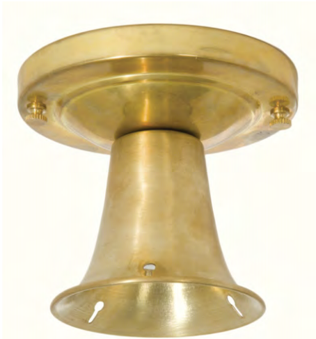
69509U - Unfinished Brass Bead Chain Fixture Hardware Set. This electrified fixture (less shade) is designed to mount onto any 3-hole bead chain glass shade. Fully assembled and ready to hang, the set comes with canopy, shade holder, porcelain socket, and 3-6" long adjustable bead chains. Approximate adjustable drop from 10" to 16". (Drop estimate includes depth of average shade). Maximum recommended bulb is 60 watts. Solid Brass, unfinished.
