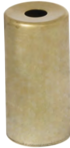
11665U - Brass socket cup, unfinished brass, 2 3/8" tall, 1.2" diameter, 1.14" inside diameter, fits E12 porcelain socket 48312 and similar-sized candelabra sockets center hole slips 1/8IP
