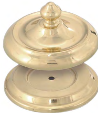
22627 - Brass three piece Handel Style heat cap set for glass dome shades, top cap 4" O.D. x 1.16" tall, inside cap is 3.9" O.D. x .41" tall, finial is .86" diameter x 1.02" tall and is tapped 1/4-27F, 6.3mm center hole on both pieces to slip 1/4-27 rod, Polished & Lacquered Finish
