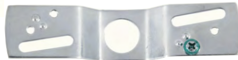
22926 - 4\frac{1}{2} " long offset crossbar, slips 3/8IP pipe, inside screw hole 2\frac{3}{4} " C to C, outside screw holes 3\frac{1}{2} " C to C, with 8-32 ground screw. Steel is .055" thick. Center hole slips 3/8 IP
