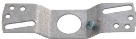
22919 - 3\frac{15}{16} " formed crossbar, 2\frac{3}{4} " to 3\frac{1}{16} " C. To C. dimension. \frac{11}{16} " center hole slip, has 8/32 ground screw. 16 gauge steel, .065" thick. Center hole slips 3/8 IP
