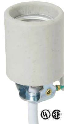
47753W- Keyless unglazed porcelain medium base (E26) socket, 1/8 IPS U-bracket hickey with strain relief, fiber sleeving, and ground wire, 8 foot 18/3 SVT white 105°C leads, aluminum screw shell, 1 1/2" O.D. x 2 1/8" height, 660W-250V
