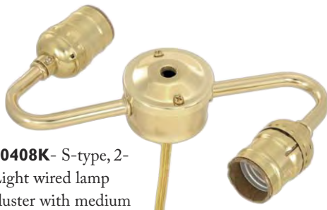
10408P - S-type, 2-Light wired lamp cluster with medium base E26 Pull Chain sockets. 7 5/8" across, 1/8F (IPS) top X 1/4F bottom with 1/8 IPS arms. Brass plated steel. 250W-250V
