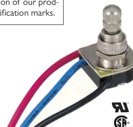
40402N - 3-Way, 4-position, 2 circuit rotary switch with nickel plated knob, load 1 on, load 2 on, load 1&2 on, off, 3/8" metal shank, 6" long 18 gauge wire leads, 3A-250VAC, 6A-125VAC, 3A,125VL
