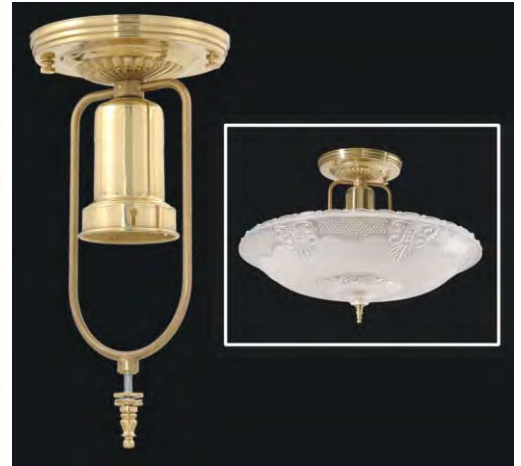
69511 - Center-Post Fixture Hardware set. This electrified fixture is designed to mount onto and hold any center-post glass fixture shade having approximately a 1/4" to 1/2" I.D. center hole. Fully assembled and ready to mount and hang, this set comes with brass canopy, socket cover and harp and porcelain socket. 10 1/2" drop from the ceiling. Solid brass, polished and lacquered finish. Use 60 watt bulb maximum. Glass shade not included. Has U.L. listed porcelain socket. Fixture is not U.L. listed.
