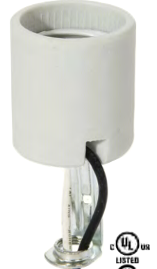
47748- Keyless unglazed porcelain medium base E26 socket with 18" 600V 150°C leads, 1/8 IPS internal extrusion single leg hickey, aluminum screw shell, 1 1/2" O.D. x 2 7/8" height, 660W-250V
