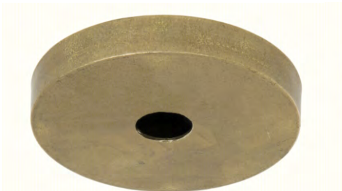
11767U - Heavy die cast brass modern style canopy, 5" diameter x \frac{3}{4} " height, 1\frac{1}{16} " I.D. center hole for screw collar loop, unfinished brass
