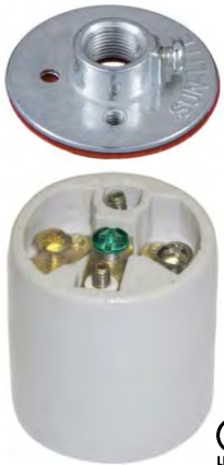
48303- E26, 660W-250V, Keyless 3-Terminal porcelain socket w/Ground Screw. Nickel plated copper screw shell. 1 1/2" O.D. x 2 1/16" ht., has metal cap with 1/8 IPS thread .
