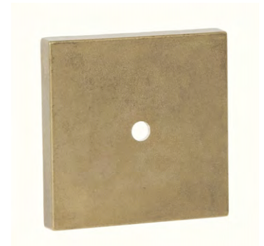
11771U - Die cast brass backplate or canopy, 3 \frac{15}{16} " square x \frac{1}{2} " deep, has a \frac{7}{16} " center hole that slips 1/8IP, fits handy box, unfinished brass
