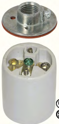
48304- E26, 660W-250V, Keyless 3-Terminal porcelain socket w/Ground Screw. Nickel plated copper screw shell. 1 1/2" O.D. x 2 1/16" ht., metal cap with 1/4 IPS thread .
