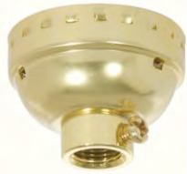
40300Gi- Socket cap with set screw, aluminum , 1/8 IPS , use w/E26 medium base electrolier socket interiors, brass plated finish
