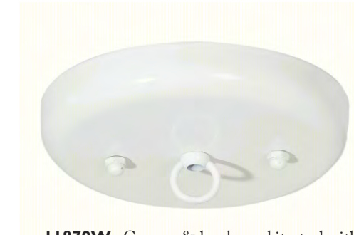
I1879W - Canopy & hardware kit, steel with WHITE finish, 5 1/4" diameter steel canopy with 1/8IP slip center hole and bar holes 2 3/4" center to center, 3/4" height. Nice, inexpensive, general purpose style canopy. Unassembled.
