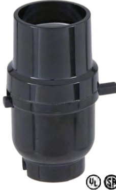
47672- Push-Thru socket, 1/8IP cap, no UNO threads, 660W-250V, 3-piece set, w/screw terminals
