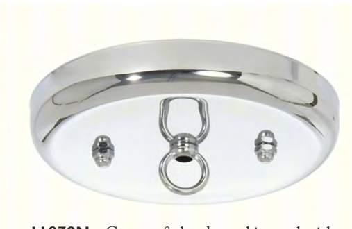
I1879N - Canopy & hardware kit, steel with NICKEL PLATED finish, 5 1/4" diameter steel canopy with 1/8IP slip center hole and bar holes 2 3/4" center to center, 3/4" height. Nice, inexpensive, general purpose style canopy. Unassembled.
