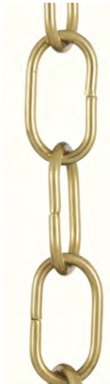
12988- Solid brass, 8 gauge machine- made oval chain (side-cut), pol- ished but not lacquered. Links are 1\frac{5}{8}" \times 1" , wire dia. .156 - Sold per yard
