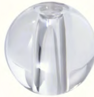
10278 -Clear acrylic spherical break, 1 1/2" diameter with 7/16" dia. center hole, all surfaces and center drill are polished clear
