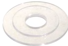
1/4" O.D., 1/16" thick, for crystal fixtures/bobesches. Seats 7/8" opening 21985 - Clear Plastic Washer 29/32" I.D.
