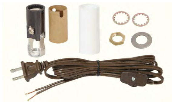
30559 - Mini-lamp kit candlestick, brown cord with line switch, comes with 1" nipple, 1/8IP hex nut and washers, 8' spt-1 brown cord, plastic candle cover, 2" candelabra (E12) lamp socket. Supplied with U.L. listed components.
