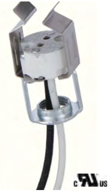
47618- Porcelain Bi-Pin halogen socket with MR-16 clip, 1/8F hickey, fits G4, G5.3, GX5.3, & G6.35, 18AWG 10" silicone/ fiberglass leads, 200°C, rated 100W-250V
