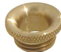
Cord Bushing 21024 - Brass, Unfinished 1/4M, 3/8" ht., 1 1/16" O.D., 1 3/32" I.D.
