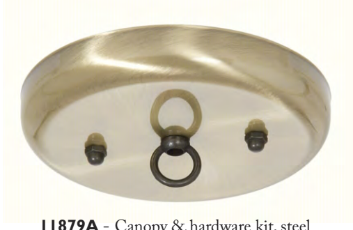
I1879A - Canopy & hardware kit, steel with ANTIQU BRASS finish, 5 1/4" diameter steel canopy with 1/8IP slip center hole and bar holes 2 3/4" center to center, 3/4" height. Nice, inexpensive, general purpose style canopy. Unassembled.
