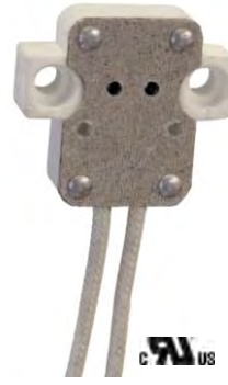
47645- Halogen socket, G5.3 with 2 mounting holes, 9" 200° SF-1 leads, 3/8" H x 1 1/16" L x 1 3/16" W, screw holes 7/8" center to center, 75W-250V
