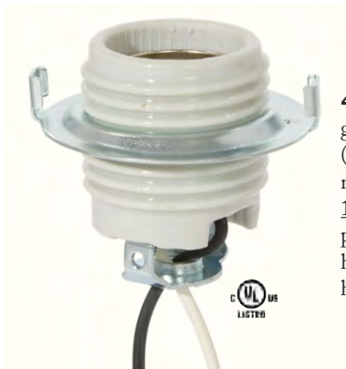
48108 - E26, 660W-250V, Medium base, porcelain screw type Keyless socket with 2 1/4" dia. threaded steel ring, insulated cap, 1/8F. Porcelain Socket has 1 1/2" outside dia. Suggested mounting hole of 1 5/8" dia. min. LEVITON Brand
