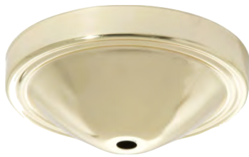
11758 - 5" diameter steel canopy, 7 / 16 " center hole slips 1/8 IP, 1 7 / 8 " tall, brass plated finish
