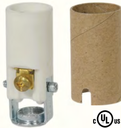
47759 - Short keyless porcelain socket, Candelabra base (E12), 1 3/4" height, Comes with a paper insulator, internal extrusion hickey is tapped 1/8IP, 75W-125V
