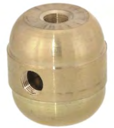
Large turned Brass 2-pc. cluster body - UNFINISHED BRASS Ht. 1 5/8", Dia. 1 1/2" Top 1/8F; Bottom 1/4F 10450 - 2 side holes 10451 - 3 side holes 10452 - 4 side holes All with 1/8F side holes
