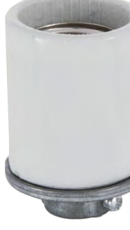
48126- E26, 660W-250V, Glazed porcelain Keyless medium base (E26) socket, high heat resistant, bottom insulator, metal 1/4 IPS cap for lamp pipe, 660W-250V. LEVITON Brand
