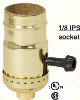
48346QC - 3-Way Turn Knob with PUSH-IN TERMINAL , 3-Way (for 3-way light bulbs) lamp socket with bright gilt finish aluminum cap & shell for standard size bulbs. Medium Base (E-26) light socket with 1/8 IPS socket cap , NO Set Screw, 250W-250V, push-in terminals with strain relief hooks.
