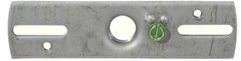
Heavy duty, galvanized plated steel crossbar bars with ground screw, .115" thick, 4 1/8" long x 1" wide, has two 8-32 tapped holes 2 3/4" center to center
