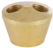
10438U - Turned Brass modern tapered body, 3/4" tall X 1 1/8" top diameter, tap 1/8F bottom and 1/8F 2 top holes , unfinished
