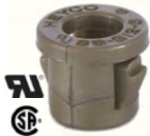
26911 - Gold snap-in cord bushing, fits a 5/16" hole for 18/2 SPT-1 cord
