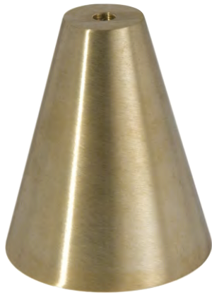
10850U - Modern conical shaped E26 medium socket cup or cast brass glass shade holder, 1 1/4" top diameter, 3 5/16" bottom diameter, 4" height, tap 1/8F center hole, unfinished brass
