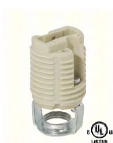
47732- G9 external threaded porcelain socket, push in terminals, 1/8IP double leg hickey (3/8" tall) with internal extrusion, 1 1/2" height, 3/4" diameter, 500W-250V - 2 AMP
