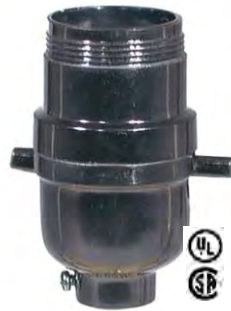
40263- E26, 660W-250V, Push-Thru phenolic shell socket with set screw in 1/8F cap and Uno threads shell. LEVITON Brand
