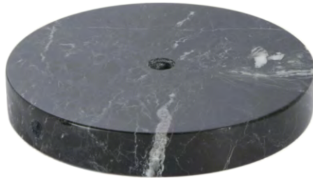
Round, black zebra marble base, ¾" thick with counter-sunk center hole that slips 1/8 IP pipe, and has a 5/16" wire way . Edges not rounded - crisp 90 degree angles.
