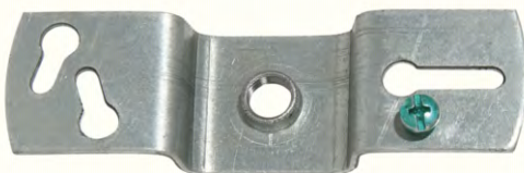
22894 - Heavy duty offset crossbar, 4\frac{3}{8} " long x 1\frac{1}{4} " wide, .08" thick, tap 1/8F middle, 8-32 ground screw inserted in hole, slotted mounting holes that will mount 2\frac{3}{4} " & 3\frac{1}{16} " center to center
