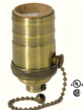
48254A- On/Off Pull Chain Heavy Turned Brass Socket with ANTIQUE BRASS Finish, On/Off Pull Chain function, NO UNO threads, 1/8IP cap with set screw, 660w, 250v
