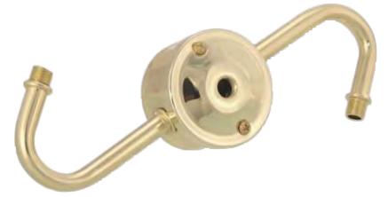
10408 - Unwired S-type, 2-Arm Lamp Cluster. 7 1/2" across, 1/8F (IPS) top X 1/4F bottom with 1/8 male IPS arms. Brass plated steel.
