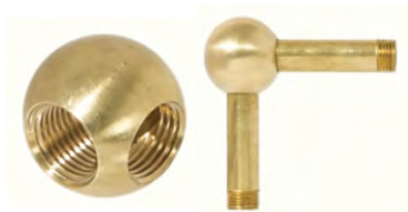
21257U - 2 Way , 7/8" diameter brass ball armback, two holes tapped 1/8F, all 90 degree, unfinished
