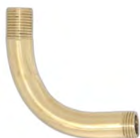
12063U- Brass bent arm, 1/8 IP tube, 1 3/4" X 1 3/4" ht. Polished, no lacquer.
