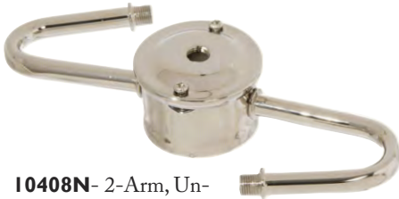
10408N - 2-Arm, Unwired lamp cluster, Nickel Plated Steel S-type, 2-Light Cluster Body. 7 1/2" across, 1/8F (IPS) top X 1/4F bottom with 1/8 IPS arms. Nickel plated steel.
