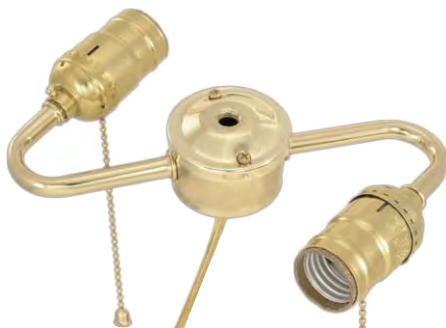
10408P - S-type, 2-Light wired lamp cluster with medium base E26 Pull Chain sockets. 7 5/8" across, 1/8F (IPS) top X 1/4F bottom with 1/8 IPS arms. Brass plated steel. 250W-250V
