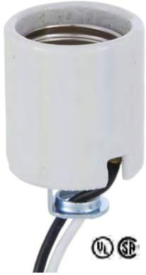
47716- Keyless unglazed porcelain medium base E26 hickey socket with 18" 105°C leads, 1/8 IPS hickey, nickel plated copper screw shell, 1 1/2" O.D. x 2" height, 660W-250V
