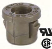
Snap-In Plastic Cord Bushing, fits a 5/16" dia. hole for 18/2 SPT-1 cord.
