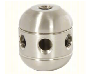
Large turned Brass 2-pc. cluster body - SATIN NICKEL FINISH Ht. 1 5/8", Dia. 1 1/2" Top 1/8F; Bottom 1/8F 10450ASN - 2 side holes 10451ASN - 3 side holes 10452ASN - 4 side holes 10448SN - 5 side holes 10453SN - 6 side holes All with 1/8F side holes
