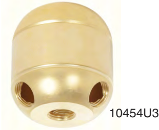
Large turned Brass 2-pc. cluster body - UNFINISHED BRASS Ht. 1 5/8", Dia. 1 1/2" Top 1/8F; Bottom 1/8F 10454U2 - 2 bottom holes 10454U3 - 3 bottom holes All with 1/8F bottom holes at 45° angle.
