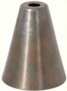
11655S - Cone shaped stamped steel socket cup for E12 candelabra sockets, 2 1/16" dia. x 2 3/8" tall, top diameter 7/8", slips 1/8IP, raw steel lightly oiled to prevent rust
