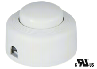
On/Off Phenolic Push Button Floor Switch, 2\frac{3}{8} " dia., for SPT-1 & SPT-2 lamp cord, rated 2A-125VAC, 1A-125VL, 1A-250VAC
