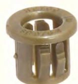
26947 - Black nylon snap-in bushing, fits a 1/2" diameter hole, fits SVT-2 and SVT-3 braided cord
