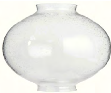
08899SEi - 9 3/4" diameter x 8" tall Onion Shade, 4" fitter each end, clear seeded glass , ground and polished top and bottom.
