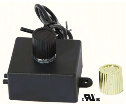
48475 - Turn-knob LED dimmer, phenolic housing, for indoor use only, comes with black and gold knobs. 2 1/4" L (including attachment points) x 1 1/2" W x 3/4" Ht. Dimmable LED 20W max, Incandescent 100W max, 120V.
