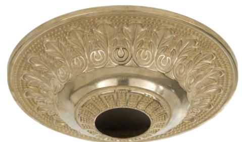
11799U - 6" Diameter, Die Cast Brass Canopy for use with screw collar loop, 6" diameter, 1 1/2" height, center hole slips 1 13/32" , accepts our screw collar loops, 10999U, 20851U, 20843U, 20827U, and 21246U, all of which are designed to support larger-size fixtures. Unfinished Brass
