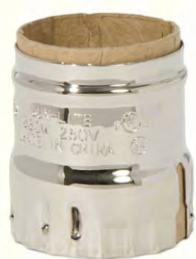
40313Ni- Short Keyless socket shell for E26 Electrolier medium size socket cap, SOLID BRASS with nickel polished & lacquered finish, no UNO threads, nickel finish
