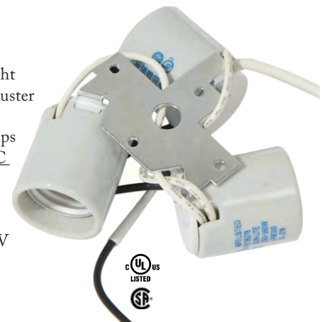
47753W- Keyless unglazed porcelain medium base (E26) socket, 1/8 IPS U-bracket hickey with strain relief, fiber sleeving, and ground wire, 8 foot 18/3 SVT white 105°C leads, aluminum screw shell, 1 1/2" O.D. x 2 1/8" height, 660W-250V
