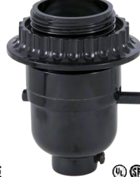
47683- Push-Thru socket, 1/8IP cap, threaded shell with ring, 660W-250V, 4-piece set, w/screw terminals
