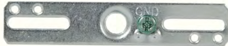
22918 - 4" Crossbar tapped 1/8F, with 8/32 Ground Screw. Slot size \frac{3}{16} " X 3\frac{5}{8} ", 16 gauge steel, .058" thick.
