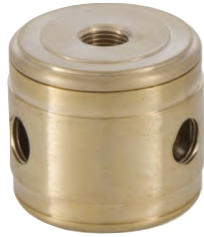
10436 - Turned Brass 2-Piece Modern Cluster Body, 1 1/2" diameter, 1 1/4" height, Top & bottom tapped 1/8F, 3 side holes tapped 1/8F, unfinished
