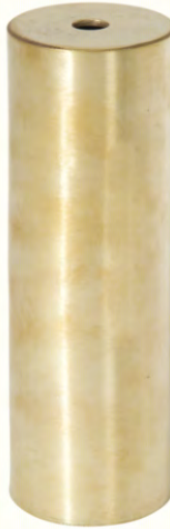
11659U - Spun brass cylinder, fits E26 medium base sockets 6 1/4" long x 2 1/16" O.D. x 2" I.D., 7/16" center hole to slip 1/8IP, unfinished
