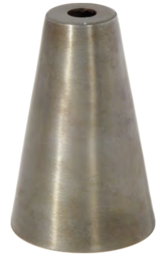
11657S - Steel cone shaped socket cup, 2.25" max O.D. x 3 3/8" tall x 1 1/16" top diameter, 7/16" center hole to slip 1/8IP, unfinished steel lightly coated in oil to prevent rust
