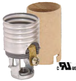
48225i- E26, 250W-250V Medium base Keyless candle socket. 2" height with 1/8F hickey & long insulator.
