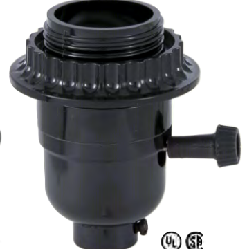
Phenolic turn-knob socket, 1/8IP cap, threaded shell with ring, 250W-250V, 4-piece set, w/screw terminals 47684- On-Off interior 47685- 3-Way interior
