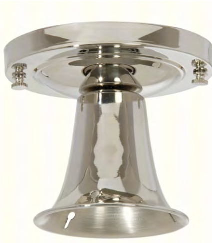
69509N - Polished Nickel Bead Chain Fixture Hardware Set. This electrified fixture (less shade) is designed to mount onto any 3-hole bead chain glass shade. Fully assembled and ready to hang, the set comes with canopy, shade holder, porcelain socket, and 3-6" long adjustable bead chains. Approximate adjustable drop from 10" to 16". (Drop estimate includes depth of average shade). Maximum recommended bulb is 60 watts. Brass, Polished Nickel Finish.
