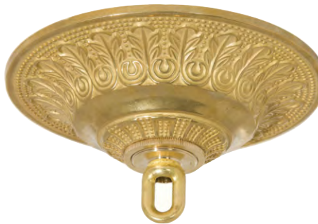
11799UK - 6" Diameter, die cast brass canopy complete with our #10999U heavy duty screw collar loop w/wire way. Comes with a heavy crossbar, ground screw, steel 1/4 IP nipple, and is 3" in height. This fine canopy is for larger-size fixtures, unfinished brass. 1 13/32" inside dia. center hole. Unassembled
