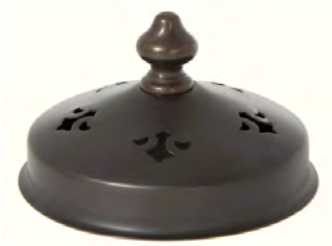
22623B - 2-Piece Handel style shade rest heat cap with flared neck to fit leaded glass shades, 3 15/16" O.D. at flare, 3 11/16" O.D. at the edge dome, 3 5/8" I.D., 2 3/4" height, finial tapped 1/4-27F, center hole slips 1/4-27 rod. Brass material with Antique Bronze Finish
