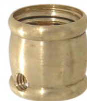
\frac{5}{8} " ht. Brass Slip coupling, \frac{5}{8} " dia. 20934 - Burn./Lacq 1/4F x 1/8IP slip with 8/32 thread side tap
