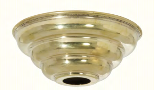
11430U - 5" diameter spun brass beehive canopy, 1 15/16" height, slips 1 1/16" center hole, unfinished
