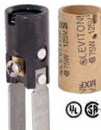
48209 - E12, 75W-125V, Candelabra base, Keyless candle socket with 1/8 F hickey & paper insulator. 3" ht. LEVITON Brand
