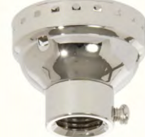
40299N- Socket cap with set screw, SOLID BRASS, 1/4 IPS, use with E26 medium base electrolier socket interiors, nickel plated finish
