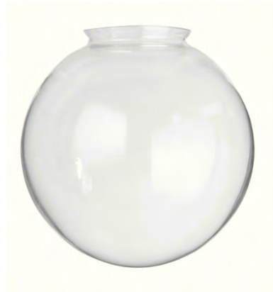
08831Ci - 4" lip fitter, 8" diameter, 8 3/16" height, closed top ball shade, clear glass, blown glass, ground and polished top.
