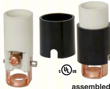
47760 - Damp location-rated short keyless porcelain socket with phenolic cover, Candelabra base (E12), 1 3/4" height, internal extrusion hickey is tapped 1/8IP, nickel plated copper screw shell, 75W-125V
