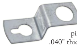
22925 - Pin-up bracket, zinc plated steel, 1 5/8" long X 5/8" wide X 1/2" offset, for pin-up lamps. Steel is .040" thick
