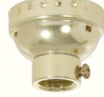
40299SG- Socket cap with set screw, aluminum , 1/4 IPS , use w/E26 medium base electrolier socket interiors, brass plated finish
