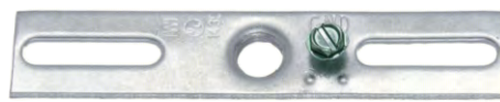
22901 - Tapped bracket bar, 3\frac{7}{8} " long, 1/8IP tap center hole, ground screw inserted. Steel is .058" thick.
