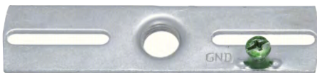
22900 - Tapped bracket bar, 3\frac{7}{8} " long, 1/4IP tap center hole, ground screw inserted. Steel is .078" thick.
