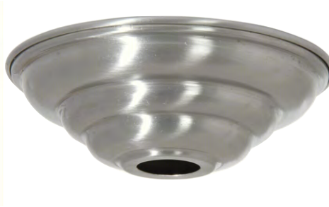
11431S - 5 1/2" diameter spun steel beehive canopy, 1 3/4" height, slips 1 1/16" center hole, raw steel.
