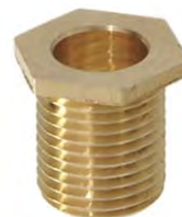
22344 - Brass Hex Nipple, 1/2" hex head, 3/8" shank, 1/2" ht., 1/8M thread
