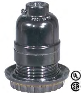
40266R- E26, 660W-250V, Keyless phenolic shell socket with 1/8F cap with set screw & threaded shell w/ring. LEVITON Brand
