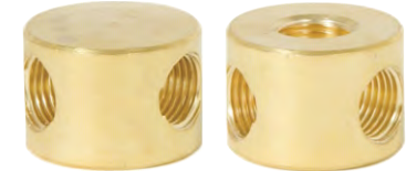
21255U - Brass straight disc arm-back, 1/4F bottom hole, 3 side holes tapped 1/4F , 1 1/4" diameter x 7/8" height, unfinished
