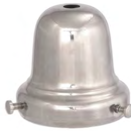
10778N - 2 1/4" Nickel Plated (brass) bell type shade holder. 2 9/16" tall, 2 1/2" actual dia. for over-sized shades.
