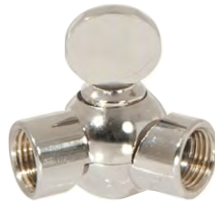
20522N - Die Cast Brass Swivel with Butterfly Knob, 3/4" diameter, 1 3 / 16 " height, 1/8F x 1/8F , Polished Nickel
