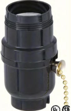
47676- Pull-Chain socket w/brass finish chain, 1/8IP cap, UNO threads, 660W-250V, 3-piece set, w/screw terminals
