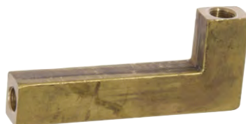
11927U- 3 3/4" long die cast brass modern style arm with wire way, 1 9/16" tall, 1/2" x 3/4" rectangular shape, tap 1/8F x 1/8F, unfinished brass
