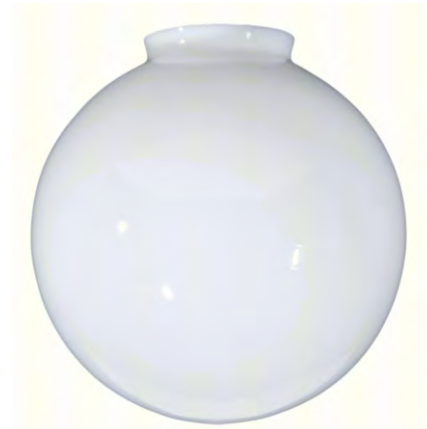
08834i - 4" lip fitter, 10" diameter, 9 5/8" height closed top ball shade, clear over opal, hand blown glass, ground and polished top.
