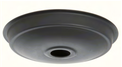
11464BK - 6\frac{1}{4} " diameter steel canopy, 1\frac{1}{16} " I.D. center hole for screw collar loop, 1\frac{1}{8} " tall, satin black finish
