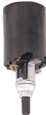
E26, 660W-250V, High heat, medium base phenolic fixture socket with On-Off bottom turn knob switch. 1 1/4" dia. body.
