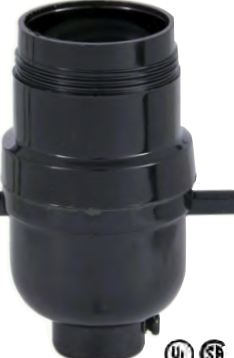
47677- Push-Thru socket, 1/8IP cap, UNO threads, 660W-250V, 3-piece set, w/screw terminals
