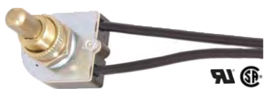
40401 - On-Off Push canopy switch with brass plated knob, 3/8" metal shank, 6" 18 gauge leads, 3A-250VAC, 6A-125VAC, 6A-125VL
