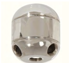
Large turned Brass 2-pc. cluster body - POLISHED NICKEL FINISH Ht. 1 5/8", Dia. 1 1/2" Top 1/8F; Bottom 1/8F 10454N3 - 3 bottom holes All with 1/8F bottom holes at 45° angle.
