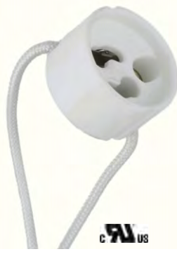
47613- Porcelain GU10 halogen socket with mounting holes, 18AWG SF-1 200°C 12" leads, rated 250W-250V, 250V/2A T-250
