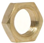
1/8F countersunk, heavy brass hex nut, 9/16" diameter, 3/16" thick, chamfered edges
