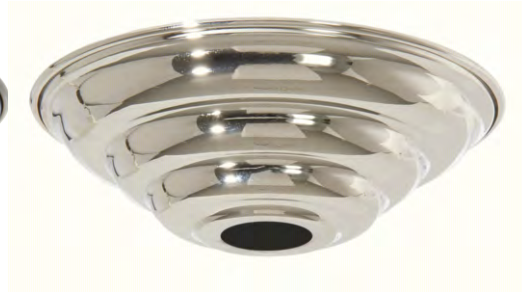
11431N - 5 1/2" diameter spun brass beehive canopy, 1 3/4" height, slips 1 1/16" center hole, polished nickel finish
