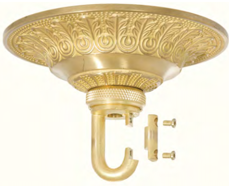
11799UB - 6" Diameter, die cast brass canopy complete with our #21246U oversized heavy duty screw collar loop w/wire way. Comes with a heavy crossbar, ground screw, steel 3/8 IP nipple, and is 4" in ht. This fine canopy is for larger-size fixtures, unfinished brass. 1 13/32" inside dia. center hole. Unassembled
