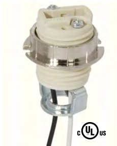
47733- G9 external threaded porcelain socket with ring, 21" UL 10362 leads rated at 600V-250°C, 1/8IP double leg hickey (3/8" tall) with internal extrusion, 1 3/8" height, 3/4" diameter, 500W-250V - 2 AMP
