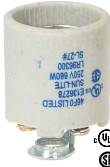
48104i- Keyless unglazed porcelain medium base (E26) socket w/detachable 1/8 IPS hickey and nickel plated copper screw shell, 1 1/2" O.D. x 2" height, 660W-250V
