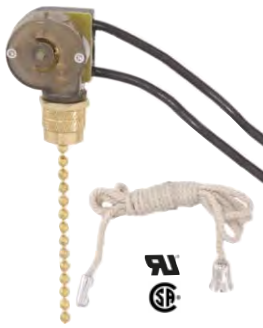
40405 - On-Off pull switch for canopy or fan light, single circuit with brass finish chain, 6" 18 gauge leads, white cord & bell, rated 3A-250VAC, 6A-125VAC
