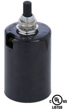
47724- Medium base E26 phenolic 2 piece bottom, On-Off turn knob husk socket, screw terminals, 1/8IP x 3/8" long bushing, 660W-250V
