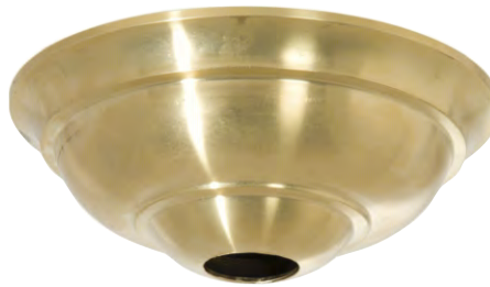
11722UH - 5 1/2" diameter unfinished brass die cast canopy, 1 3/4" height, has 1 1/16" diameter hole for screw collar loop, unfinished brass
