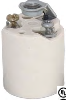
48104- E26, 660W-250V, Medium based Keyless porcelain fixture socket with 1/8 IPS detachable hickey. Has high heat resistant quality. LEVITON Brand
