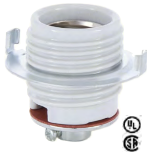
47705 - Medium base E26 threaded Keyless porcelain socket with metal ring, has terminal screws, 1/8 IPS cap with set screw, nickel plated copper screw shell. Porcelain Socket has 1 1/2" outside dia., 660W-250V
