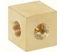
21274U - Brass 90 degree armback, tapped 1/8F x 1/8F, 7/8" x 7/8", Unfinished Brass
