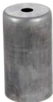
11662S - Metal socket cup, unfinished steel, 3" tall, 1⅝" diameter, 1⅞" inside diameter, fits E26 (medium) sockets 48101, 48104, & 48105, center hole slips 1/8IP
