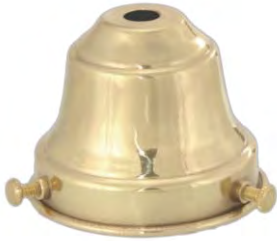
10763U - Unfinished Spun Brass Fixture Shade Holder for 2 1/4" fitter shades. 2 5/8" deep w/rolled edges & 3 screw eyelets. Slips 1/8 IP.
