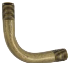
12069U- Brass Bent Arm, 2" x 2", 1/8M X 1/8M, unfinished brass
