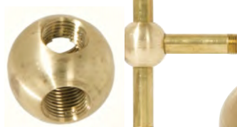
21259U - 3 Way , 7/8" diameter brass ball armbak, three holes tapped 1/8F, unfinished
