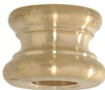
5/8" ht. Brass Neck, 15/16" dia. Unfin. 20980 - Slips 1/8 IP 20981 - Tap 1/8 F
