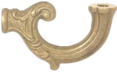
11969U - 3 7/8" L. X 2 3/8" ht. die cast brass arm with internal wire way, tapped 1/8F X 1/8F. Unfinished
