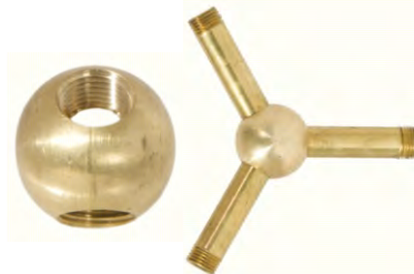
21258U - 3 Way , 7/8" diameter brass ball armback, three holes tapped 1/8F, all 120 degree, unfinished
