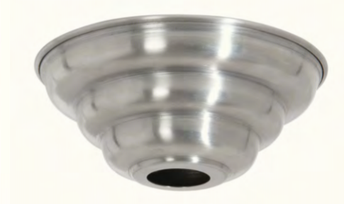
11430S - 5" diameter spun steel beehive canopy, 1 15/16" height, slips 1 1/16" center hole, raw steel.
