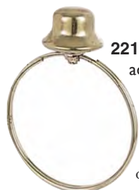
22114 - Shade Adapter. Brass finish. Converts washer type shade to fit on regular shape bulb. 1/4-27M.
