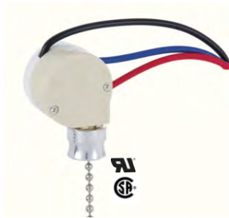
40412 - 3-Way ceiling fan canopy switch, two circuit with nickel finish chain, 6" 18 gauge leads, white cord & bell, rated 6A-125V, 3A-250V
