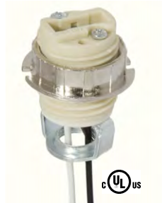
47734- G9 external threaded porcelain socket with ring, 72" UL 10362 leads rated at 600V-250°C, 1/8IP double leg hickey (3/8" tall) with internal extrusion, 1 3/8" height, 3/4" diameter, 500W-250V - 2 AMP
