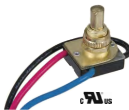
40409 - 3-Way, 4 position, push canopy switch with brass plated knob, 3/8" metal shank, 6" 18 gauge leads, 3A-250VAC, 6A-125VAC
