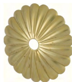
11522U- Stamped brass bobesche, 5/16" tall x 2 15/16" O.D., slips 1/8 IP, Unfinished brass
