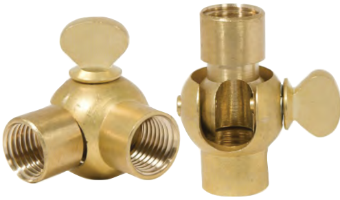
20548U - Die Cast Brass open ball Swivel with key, 1 11 / 16 " long x 1 1 / 2 " ht, x 7/8" wide, Tapped 1/4F X 1/4F , unfinished
