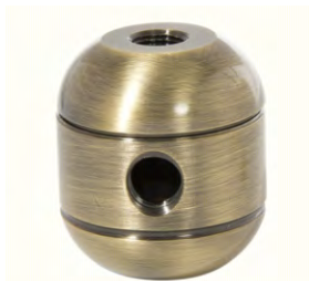
Large turned Brass 2-pc. cluster body - ANTIQUÉ BRASS FINISH Ht. 1 5/8", Dia. 1 1/2" Top 1/8F; Bottom 1/8F 10450AA - 2 side holes 10451AA - 3 side holes 10452AA - 4 side holes 10448A - 5 side holes All with 1/8F side holes
