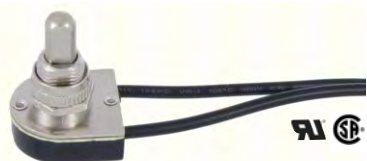
40401N - On-Off Push canopy switch with nickel plated knob, 3/8" metal shank, 6" 18 gauge leads, 3A-250VAC, 6A-125VAC, 6A-125VL
