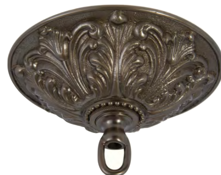
11877B- Die Cast Brass Canopy, 5 1/2" dia., 3 3/8" deep, with 1 1/16" center hole with screw collar loop and ceiling hard- ware, antique bronze finish
