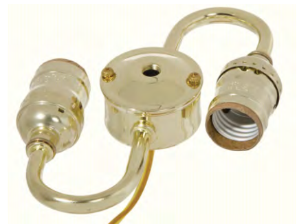
10429 - 2-Light wired lamp cluster with medium base E26 Keyless Sockets 7" across, 1/8F (IPS) top X 1/8F bottom with 1/8 IPS arms. Steel with Brass Plated finish. All U.L. recognized components, but unit not U.L. listed
