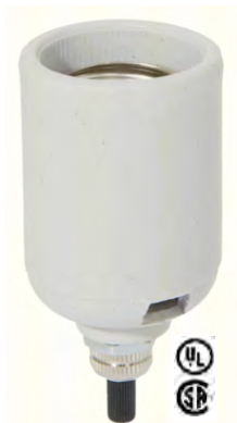
47724P - Unglazed porcelain socket w/bottom turn knob, nickel plated E26 copper screw shell, has screw terminals. 1/8M x 3/8" long shank. 660W, 250V
