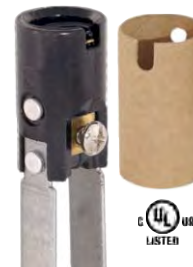
48209i - E12, 75W-125V, Candelabra base, Keyless candle socket with 1/8 F hickey & paper insulator. 3" ht.
