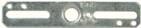
22911 - 4" crossbar tapped 1/8F w/ 8/32F Gnd. Hole. Slot size \frac{3}{16} " X 3\frac{5}{8} ", 16 gauge steel, .063" thick. No ground screw
