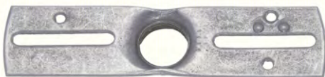
22923 - 4\frac{3}{16} " long cross bar, tap 3/8IP, 8/32 ground hole (no screw inserted). Steel is .075 thick
