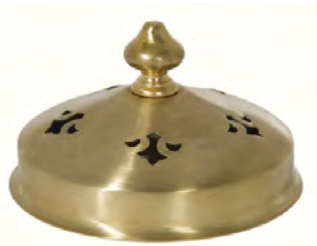
22623U - 2-Piece Handel style shade rest heat cap with flared neck to fit leaded glass shades, 3 15/16" O.D. at flare, 3 11/16" O.D. at the edge dome, 3 5/8" I.D., 2 3/4" height, finial tapped 1/4-27F, center hole slips 1/4-27 rod. Unfinished Brass
