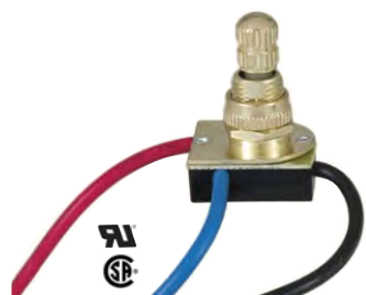
40402i - 3-Way, 4-position, 2 circuit rotary switch with brass plated knob, load 1 on, load 2 on, load 1&2 on, off, 3/8" metal shank, 6" long 18 gauge wire leads, 3A-250VAC, 6A-125VAC, 3A,125VL
