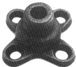
22913 - 3/8M X 1/8F Iron Fixture Stud for heavy duty use. 1" ht., 1 3/4" square with 1/4" dia. mounting holes.
