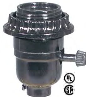
40264R- E26, 250W-250V, Regular ON-Off Turn Knob phenolic shell socket with 1/8F cap with set screw & threaded shell w/ring. LEVITON Brand
