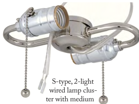
S-type, 2-light wired lamp cluster with medium base E26 Pull Chain sockets, 1/8F (IPS) top X 1/8F bottom, 14" 18/2 SPT-2 105°C lamp cord. Choice of finish. 250W-250V 10412N - Nickel plated finish, clear silver cord 10412 - Brass plated finish, clear gold cord
