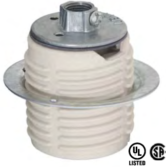
48108 - E26, 660W-250V, Medium base, porcelain screw type Keyless socket with 2 1/4" dia. threaded steel ring, insulated cap, 1/8F. Porcelain Socket has 1 1/2" outside dia. Suggested mounting hole of 1 5/8" dia. min. LEVITON Brand
