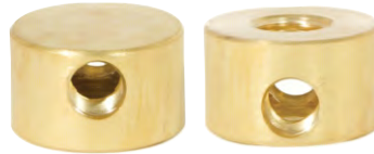
21250U - Brass straight disc arm-back, 1/4F bottom hole, 2 side holes tapped 1/8F , 1 1/4" diameter x 3/4" height, unfinished
