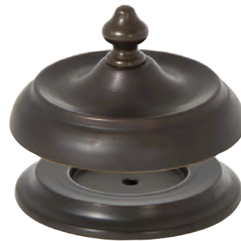
22627B - Brass three piece Handel Style heat cap set for glass dome shades, top cap 4" O.D. x 1 1/2" tall, inside cap is 3 7/8" O.D. x 7/16" tall, finial is tapped 1/4-27F, center hole slips 1/4-27 rod, Antique Bronze Finish
