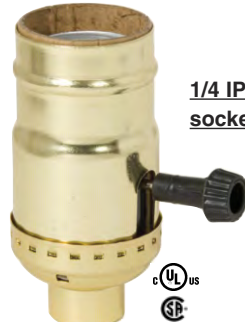
48349QC - 3-Way Turn Knob with PUSH-IN TERMINAL , 3-Way (for 3-way light bulbs) lamp socket with bright gilt finish aluminum cap & shell for standard size bulbs. Medium Base (E-26) light socket with 1/4 IPS socket cap , NO Set Screw, 250W-250V, push-in terminals with strain relief hooks
