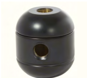
Large turned Brass 2-pc. cluster body - SATIN BLACK FINISH Ht. 1 5/8", Dia. 1 1/2" Top 1/8F; Bottom 1/8F 10450ABK - 2 side holes 10451ABK - 3 side holes 10452ABK - 4 side holes 10448BK - 5 side holes 10453BK - 6 side holes All with 1/8F side holes
