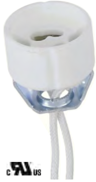
47612- Porcelain GU10 halogen socket with 1/8IP hickey, 18AWG SF-1 200°C 12" leads, rated 250W-250V, 250V/2A T-250
