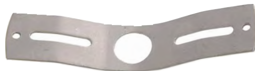
22910 - 4\frac{5}{8} " Offset Crossbar, slips over \frac{5}{8} " dia. stud. 8/32 tapped holes are 4\frac{1}{4} " C. to C., no ground hole. Steel is .060 thick. Center hole slips 3/8 IP
