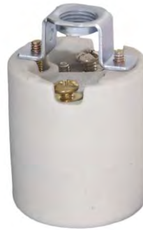
48301- E26, 660W-250V, Heavy duty, medium base, unglazed porcelain Keyless socket. Aluminum screw shell. Has approx. 5/8" ht. detachable, 1/8 IPS hickey.
