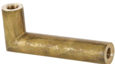
11928U- 3 3/4" long die cast brass modern style arm with wire way, 1 9/16" tall, 3/4" diameter (round shape), tap 1/8F x 1/8F, unfinished
