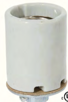
47754- Keyless glazed porcelain medium base (E26) socket, 1/8 IPS metal cap with set screw, nickel plated copper screw shell, 1 1/2" O.D. x 2 1/16" height, 4KV pulse rated , 660W-600V
