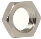
1/8F countersunk, heavy brass hex nut, 9/16" diameter, 3/16" thick, chamfered edges
