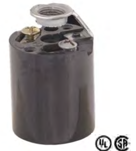
48101- E26, 660W-250V, Medium base, Keyless phenolic fixture socket w/detachable hickey tapped 1/8F. (1 7/8" overall ht.). LEVITON Brand
