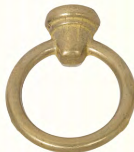
2" diameter, 2 5/16" ht. Heavy Cast Brass Loop, NO wire way, tap 1/8F, unfinished 21194U - Unfinished Tap 1/8F
