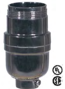
40266- E26, 660W-250V, Keyless phenolic shell socket with set screw in 1/8F cap and Uno threads shell. LEVITON Brand
