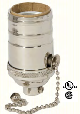
48254N- On/Off Pull Chain Heavy Turned Brass Socket with POLISHED NICKEL Finish, On/Off Pull Chain function, NO UNO threads, 1/8IP cap with set screw, 660w, 250v
