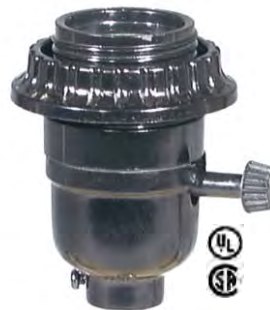
40265R- E26, 250W-250V, 3-Way phenolic shell turn knob socket with 1/8F cap with set screw and threaded shell with ring. LEVITON Brand
