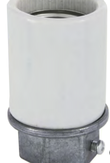
48125- E26, 660W-250V, Glazed porcelain Keyless medium base (E26) socket, high heat resistant, bottom insulator, metal 1/2 IPS cap for lamp pipe, 660W-250V. LEVITON Brand
