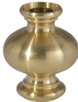
2 5/16" ht. Brass Column, 1 7/8" dia., seats 1" top, seats 1" bottom 10430U - Unfinished Slips 1/4 IP
