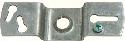
22893 - Heavy duty offset crossbar, 4\frac{3}{8} " long x 1\frac{1}{4} " wide, .08" thick, tap 1/4F middle, 8-32 ground screw inserted in hole, slotted mounting holes that will mount 2\frac{3}{4} " & 3\frac{1}{16} " center to center
