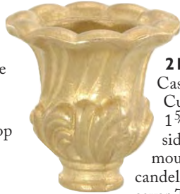
21800U - Unfinished Die Cast Brass Candle Cup, 2 3/8" ht., 1 1/2" O.D., 1" inside top opening. mounts standard or candelabra candle cover, tap 1/8F.
