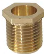
22359 - Brass Small Head Flange Nipple, 13/32" hex head, 3/8" shank, 1/8M thread
