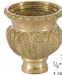
21804U - Die Cast Brass Candle Cup, 1 5/8" ht., 1 5/8" O.D., 1" inside top opening, mounts standard or candelabra candle cover. Tap 1/8F. Unfin.
