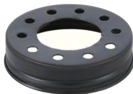
20051BK- Steel mason jar lid with 1.40" diameter center hole to fit E26 phenolic pendant socket with ring (not included). 10 air vent holes (.22" diameter), 2 7/8" O.D., satin black finish .
