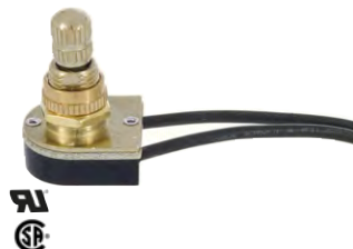
40400i - On-Off Rotary canopy switch with brass plated knob on 3/8" metal shank, and 6", 18 ga. wire leads. Rated at 3A-250-VAC, 6A-125VAC, 6A-125VL
