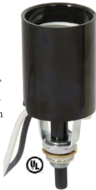
47747- E26 Medium Base Phenolic Socket with bottom turn knob , 13" AWM B/W 105° Leads, 1/8M bottom bushing with nut, 1 1/4" diameter x 2 3/8" height to bottom of hickey, 2 3/4" overall height, 660W - 250V
