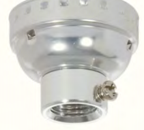
40299SN- Socket cap with set screw, aluminum , 1/4 IPS , use with E26 medium base electrolier socket interiors, nickel plated finish
