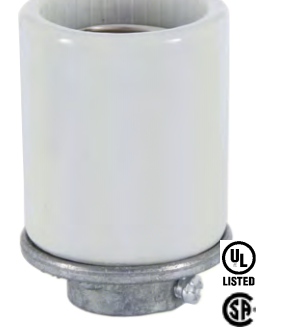
48105C- E26, 660W-250V, Glazed porcelain Keyless medium base (E26) socket, high heat resistant, bottom insulator, metal 3/8 IPS cap for lamp pipe, 660W-250V, LEVITON Brand
