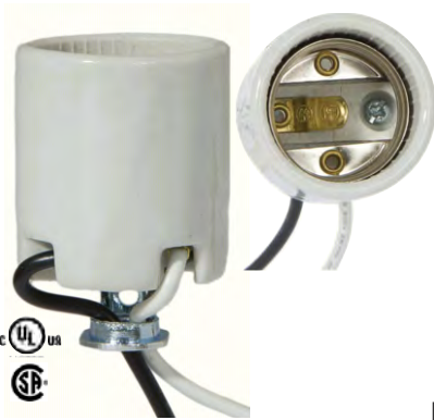
Keyless glazed porcelain, E26 med.base lamp socket with 1/8 IPS hickey, 105°C 600V lead wires, and nickel plated copper screw shell. 1 1/2" O.D. x 2" height, 660W-250V. Your choice of wire leads length.
