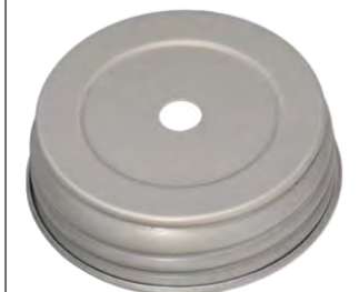
20014- Heavy Zinc Mason jar adapter. May be completed w/socket cap no. 40102N & clear silver lamp cord no. 46703 or 46713 for a great looking adapter. 2 1 / 16 " I.D. base, top hole slips 1/8 IP.
