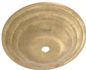
10838U - Die cast brass canopy or back plate, 4 3/4" X 1 1/8", with 1/8 IP slip hole. Unfinished brass
