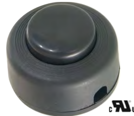
On/Off Phenolic Push Button Floor Switch, 2\frac{3}{8} " dia., for SPT-1 & SPT-2 lamp cord, rated 2A-125VAC, 1A-125VL, 1A-250VAC
