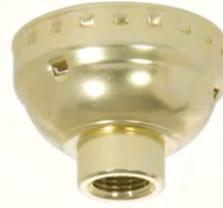
40303SGi- Socket cap less set screw, aluminum , 1/8 IPS , use w/E26 medium base electrolier socket interiors, brass plated finish
