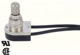
40400N - On-Off Rotary canopy switch with nickel plated knob, 3/8" shank, 6" 18 gauge leads, 3A-250VAC, 6A-125VAC, 6A-125VL
