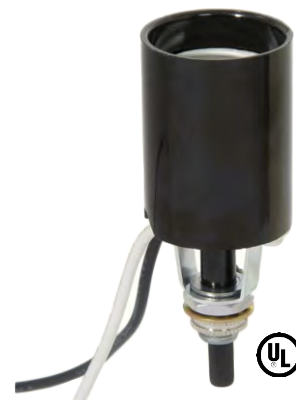
47747 - E26 Medium Base Phenolic Socket with bottom turn knob , 13" AWM B/W 105° Leads, 1/8M bottom bushing with nut, 1 1/4" diameter x 2 3/8" height to bottom of hickey, 2 3/4" overall height, 660W - 250V
