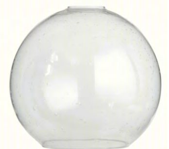
08860SEi - Hand blown clear seeded glass ball shade, 7 7/8" diameter, 7 1/16" tall, top center hole is 1.65" I.D., bottom center hole is 4.25" O.D., fits our socket cover 11656 series, ground and polished top & bottom. SEE ILLUSTRATION ABOVE!
