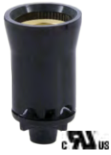
47725 - Pin type phenolic E12 candelabra base socket, pressure fit, 1 1/4" ht., 3/4" dia. 60W-125V
