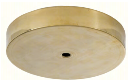
10051U - 5" dia. Modern style SPUN BRASS base, 1/8F (7/16" dia) center hole, 1" ht. Bottom with rolled in edge.
