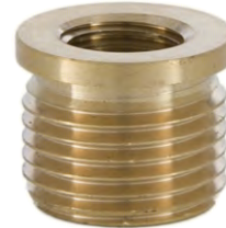
Shoulder Reducer 21145U - Brass, Unfin. 1/2M X 1/4F
