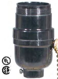
40262- E26, 660W-250V, On-Off Pull Chain phenolic shell socket with set screw in 1/8F cap and Uno threads shell. LEVITON Brand
