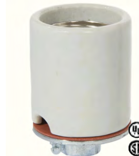
47755- Keyless glazed porcelain medium base (E26) socket with side wire ways , 1/8 IPS metal cap with set screw, nickel plated copper screw shell, 1 1/2" O.D. x 2 1/16" height, 660W-250V
