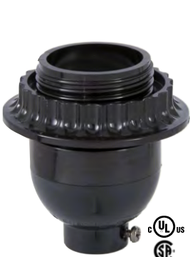
47687- Short Keyless socket, 1/8IP cap, threaded shell w/ring, 660W-250V, 4-piece set, w/screw terminals, can be used with 20050 series jar lids & neckless glass holders
