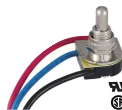
40409N - 3-Way, 4 position, push canopy switch with nickel plated knob, 3/8" metal shank, 6" 18 gauge leads, 3A-250VAC, 6A-125VAC
