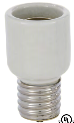
48711 - Mogul to mogul socket extension, 2 3/8" overall extension, 4KV pulse rating, 1500W-600V, E39-E39
