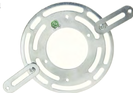
22891 - 4" universal circle crossbar with mounting wings, ground screw, wings let you extend the crossbar from 4" to 6\frac{1}{4} " center to center. Steel is .056" thick
