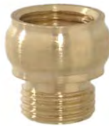
Turned Brass Beaded Nozzle, 17/32" dia., 9/16" ht. 20941U - Unfin. 1/8F x 1/8M
