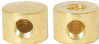
21253U - Brass straight disc arm-back, 1/4F bottom hole, 1 side hole tapped 1/4F , 1 1/4" diameter x 7/8" height, unfinished brass
