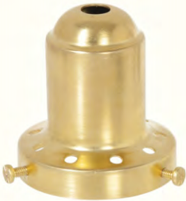
Vented Fixture Shade Holder for 2 1/4" fitter shades. 2 5/8" ht., 2 7/16" outside dia. Slips 1/8 IP.
