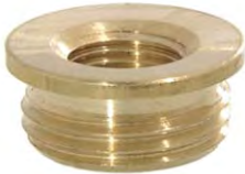
Brass Reducer, 3/4" dia., 11/32" ht. 20943 - Unfin. 1/8 F x 3/8 M
