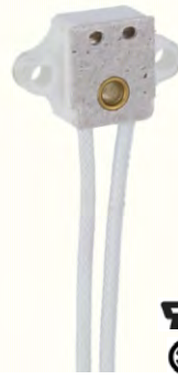
47617- Porcelain Bi-Pin halogen socket, fits G4, G5.3, GX5.3, & G6.35, 18AWG 10" silicone/ fiberglass leads, 200°C, rated 100W-250V
