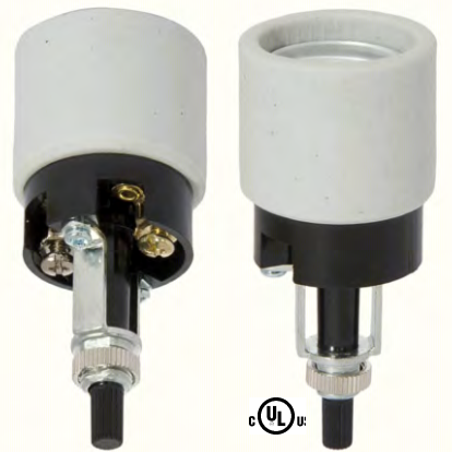
47651 - Medium base E26 phenolic and unglazed porcelain shell socket w/bottom turn-knob, hickey with 1/8M (3/8" long) nipple, screw terminals, 1 1/2" diameter, 3 1/4" overall height, 2 1/2" from top to bottom of hickey, 660W-250V
