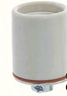
48302- E26, 660W-250V, Glazed porcelain Keyless medium base socket with high heat resistance. Has bottom insulator, 1/8 IPS , aluminum screw shell, metal cap & set screw.
