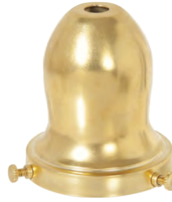
10853U - Brass Holder, 2 1/4" Fitter, 3" Height with Set Screws, Slips 1/8 IPS, Three 8-32 Eyelets, unfinished, 2 11/16" O.D. x 2 5/16" I.D.
