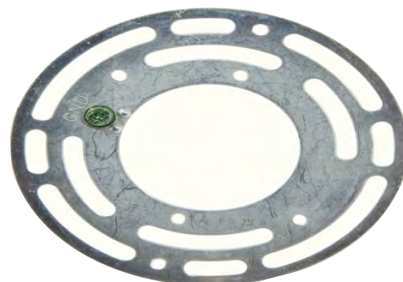
22885 - Steel Universal Circle Crossbar, 1\frac{13}{16} " center hole - 4" O.D., 2\frac{1}{8} " C to C, 2\frac{3}{4} " C to C, 3\frac{1}{2} " C to C. With ground screw. Steel is .056" thick
