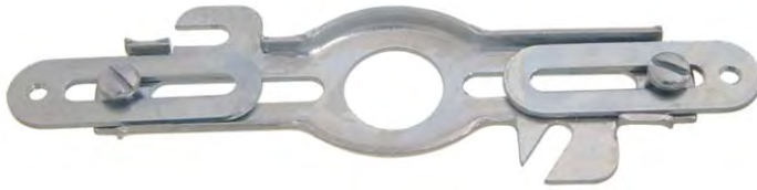
22927 - 4" universal cross bar, slips 3/8IP, inside screw holes 2 3/4" C to C, outside screw holes 3 9/16" C to C, tapped 8/32, 8/32 ground hole (no screw inserted). 16 gauge steel, .065" thick. Center hole slips 3/8 IP
