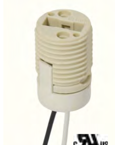
47735- G9 external threaded phenolic socket, 20" UL 10362 leads rated at 600V-250°C, 1/8F bushing, 1 1/4" height, 3/4" diameter, 500W-250V - 2 AMP
