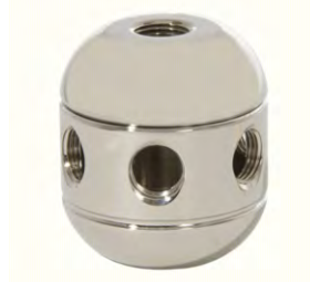
Large turned Brass 2-pc. cluster body - POLISHED NICKEL FINISH Ht. 1 5/8", Dia. 1 1/2" Top 1/8F; Bottom 1/8F 10450AN - 2 side holes 10451AN - 3 side holes 10452AN - 4 side holes 10448N - 5 side holes 10453N - 6 side holes All with 1/8F side holes
