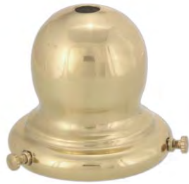
10751U - 2 1/4" fitter, spun brass, bulbous shaped shade holder, 2 9/16" ht. X 2 3/4" dia., slips 1/8IP. No key slot, Unfinished Brass
