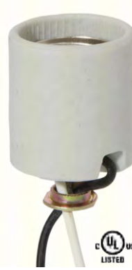
47745- Keyless unglazed porcelain medium base E26 socket with 18" 600V, 150°C leads, 1/8 IPS hickey, nickel plated copper screw shell, 1 1/2" O.D. x 2" height, 660W-250V
