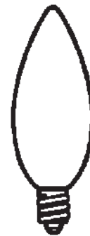
CT Candelabra base, Torpedo Tip Decorative bulb, 32 mm, 3000 hrs.
