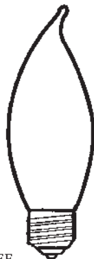
EF Standard base, Flame Tip Decorative bulb, 3000 hrs.
