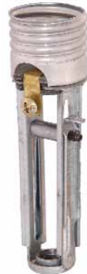
48208i- Standard base, adjustable keyless candle socket. Ht. adjusts from 4" to 5 3/4" & comes w/a long paper insulator. 250V-660W UL CSA, Imported
