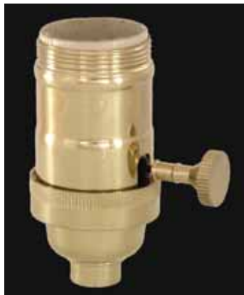
48240- Polished & Lacquered Brass, 3-way heavy duty, solid turned brass socket with heavy turn knob, uno threads, and U.L. listed, medium base interior. Has 1/8F base with set screw.
